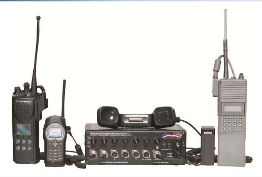
The Incident Commanders' Radio Interface (ICRI) brings multiple tools to improve radio communications --- enhancing in-building operation, and improving warfighter and first responder safety in buildings, subways, and areas with unreliable radio coverage.
